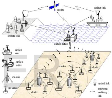
Three-dimensional UW-ASNs for ocean column monitoring. These include networks of sensors whose depth can be controlled, and may be used forsurveillance applications or monitoring of ocean phenomena (ocean bio-geo-chemical processes, water streams, pollution, etc).
